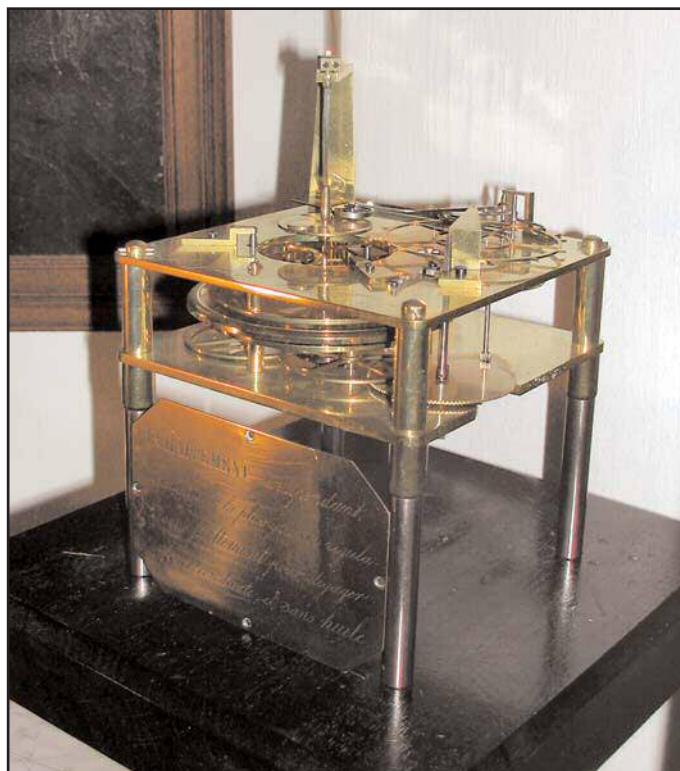
Figure 2. Clockwork escapement by Ludovic Gavioli, 1830. The main spindle is supported laterally by three large wheels, thus reducing friction (ball bearings were not known at this time). From the collection of the Museum Speelklok tot Pierement, Utrecht. Photo: KDV.
